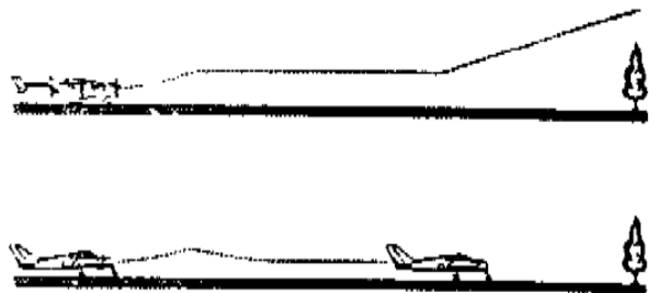
Fig. 7 - Take-off profile with engine cut at 1.1 V_5
